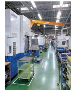
Small batch production line for torque converters
